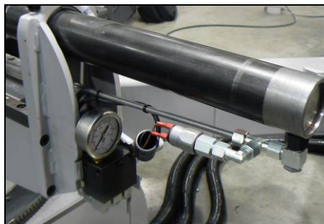
Pressure in main vice – manometer is placed on main vice
