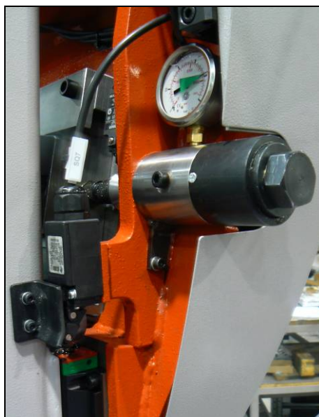
Saw blade tensioning – placed on saw arm.
