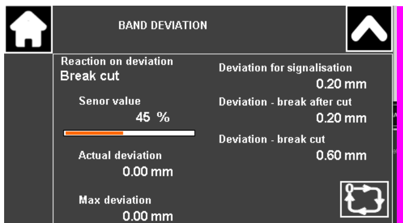
Screen with viewing the parameters of the band deviation
