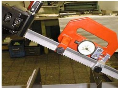
3. Stretch the saw band until it is stretched to the recommended value
