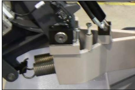
Setting the lower stop position is set using the screw in Console.
