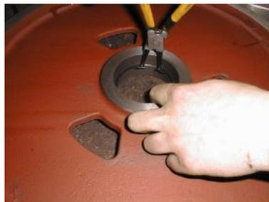
7. Insert the retaining ring to the hole in the wheel.
