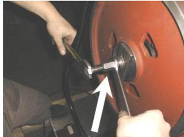
5. Screw on the preparation to the wheel stretching to the hole in the shaft. Pull on the wheel on the shaft.
