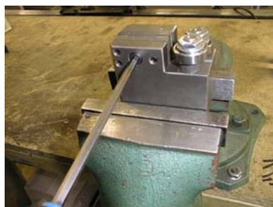
3. Loosen the binding screw of first metal guide. Remove adjustable hard metal guide.
