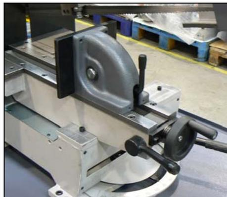
Release the clamping lever, shift the vice ca. 5 mm from the material and clamp the material to the vice by lever.
