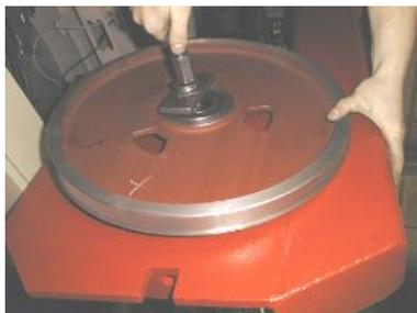
9. Put the wheel on the shaft and screw on the preparation to the wheel stretching to the hole in the shaft.
