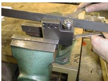
9. Insert the saw band to the guiding cube (ca. 15 – 20 cm). Set the eccentrics by means of the wrenches, the saw band must run in the centre. Guide pulleys must not press too much on the band, but must spin freely during the band run.
