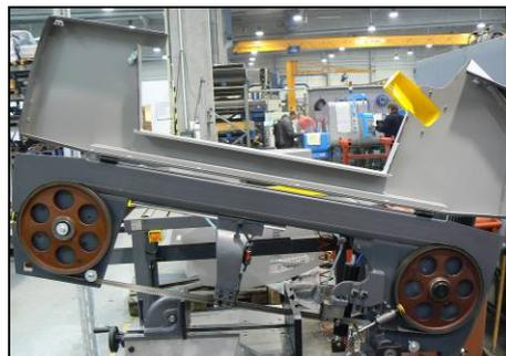
**The band saw is stated to the operation, when the covers is closed!** Limit switche on saw arm control if covers are open or not.
