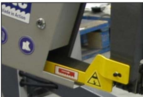
Never switch on the saw band drive if this cover is not mounted!
