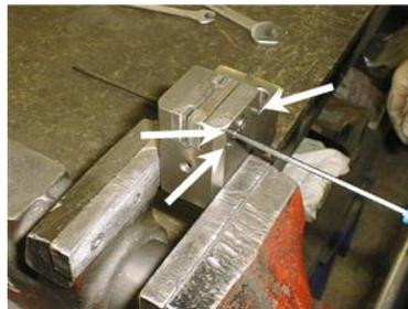
2. Loosen the adjusting screws of the metal guide.
