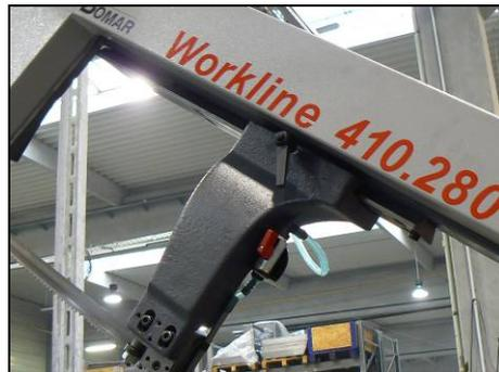
1. Release the stopping lever of the listel. Move the left part of the guide so that the left edge of the guide blocks is as close as possible cutted material.
