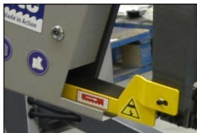
2. Dismantle yellow protective cover of the saw band. The cover is clamped with two screws.
