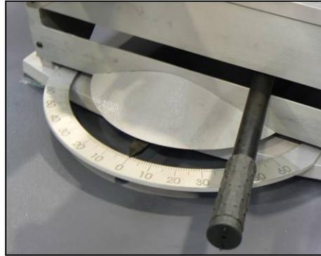
1. Release securing lever of the console, Swivel the frame to the desired angle by pulling the saw arm. Angle is shown on scale. a páku znovu utáhněte. Then re-tighten the lever.
